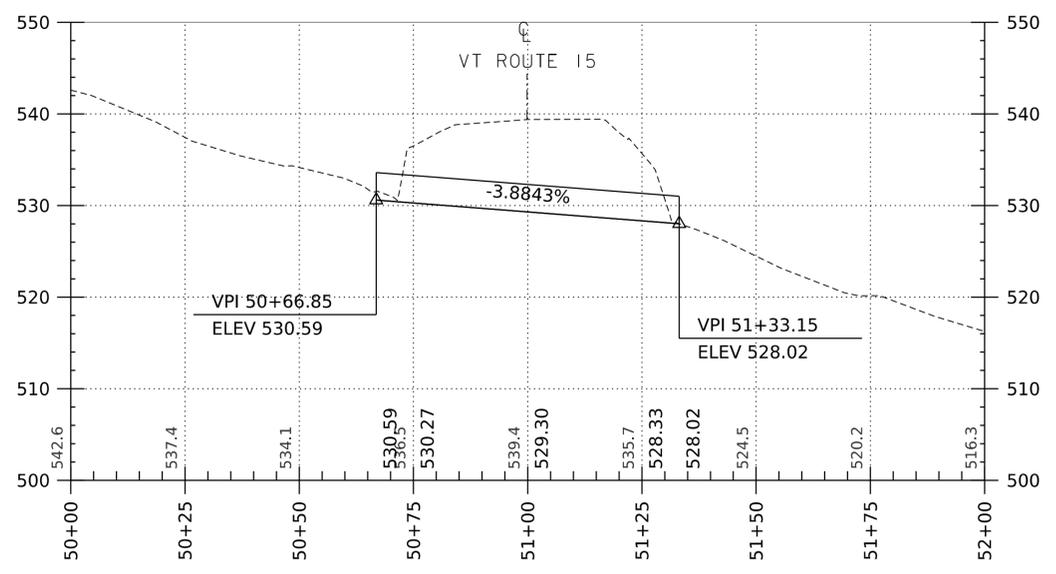
**CULVERT 6A NEW CULVERT CHANNEL PROFILE**
